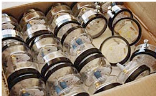
HANDY LIGHT: Residents of Tahana received LED lamps for their homes, churches, and school. Each lamp has a dozen white LEDs that fit into a transparent plastic case.
