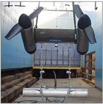
SMD Hydrovision will soon make a full-scale version of this prototype tidal energy device.
