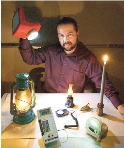
EETD's Evan Mills holds his prototype white-light-emitting diode (WLED) made by a company called Ignite Innovations.
