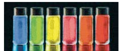
Quantum dots of the same material but different sizes have different band gaps and emit different colors.
