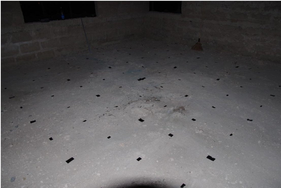
4 * 4 meters on-location grid for illumination measurements
