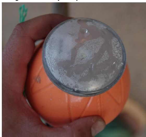
Figure 16. Trony Lamps with water inside
