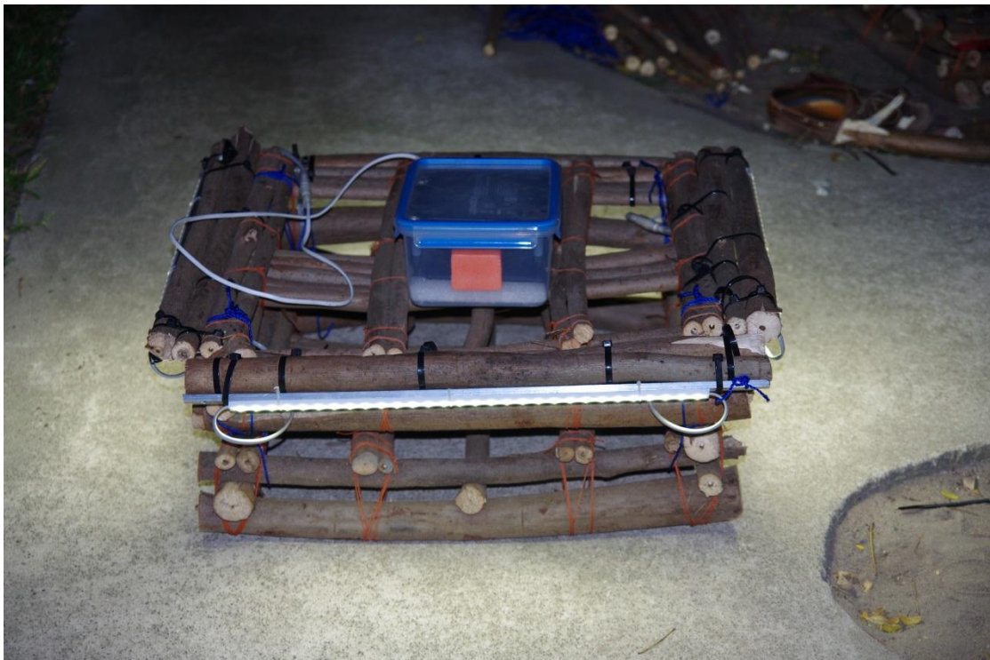
Configuration 6: Lumintronix Superflux LED strips: 4 strings, white, user-improved
