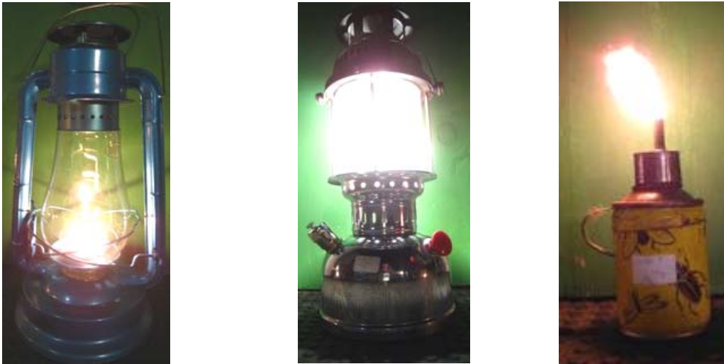
Figure 4. Kerosene lamps used by small businesses in Maai Mahiu and Karagita, Kenya: hurricane-style, pressure-style, and wick lamp (from left to right)
