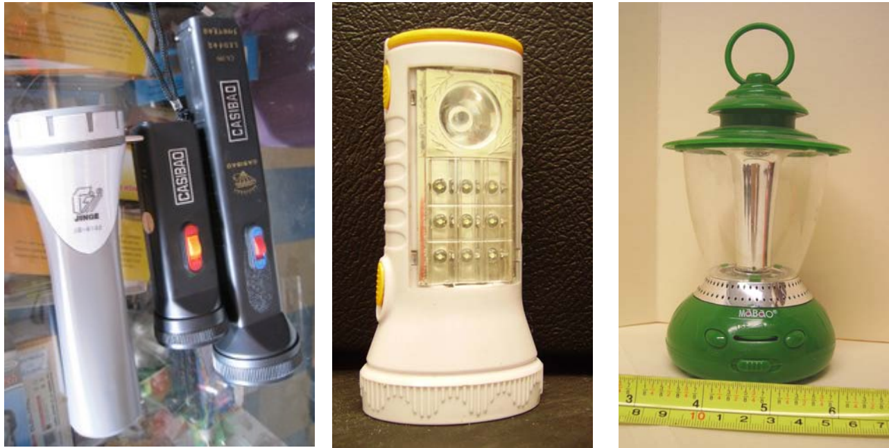
Figure 7. LED flashlights shown in a shop in Naivasha Town market (left), an LED torch with integrated LED array purchased in Karagita market (middle), and an LED lantern-style lamp with an integrated radio feature purchased in Karagita market (right)
