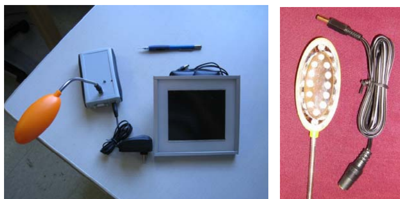
Figure 8. Image of the LED-based lighting kit offered to businesses during the study. The one Watt solar module was available as an optional charging source. The pen included is for scale. A close up of the lamp head and six foot long extension cable for the lamp are shown on the right.
