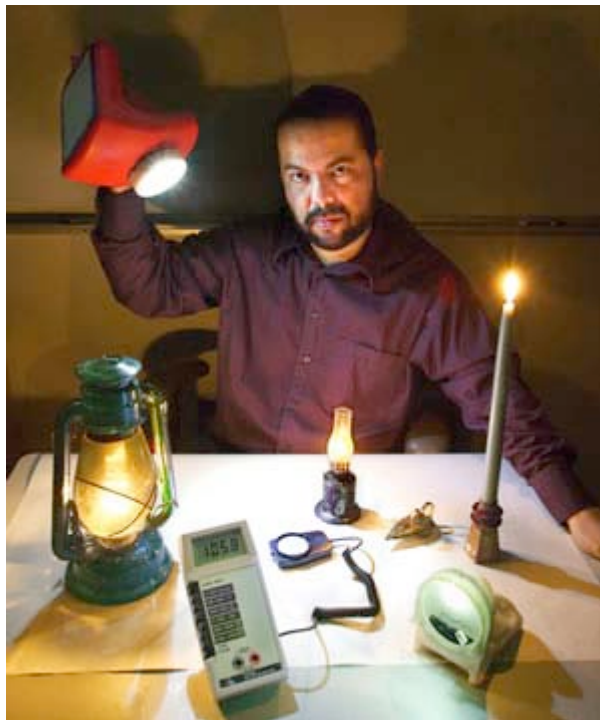
Evan Mills, an energy efficiency expert, holds a prototype white light-emitting diode (WLED) made by a company called Ignite Innovations. This lamp, which grew out of a Stanford-led effort involving several Silicon Valley companies, Berkeley Lab, and others, features a one watt WLED, solar panel and rechargeable AA batteries. (Photo by Roy Kaltschmidt)
