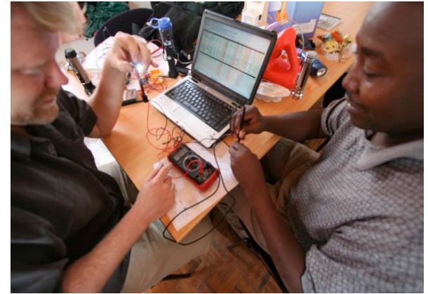
Measuring current draw for LED lights in Kenya
