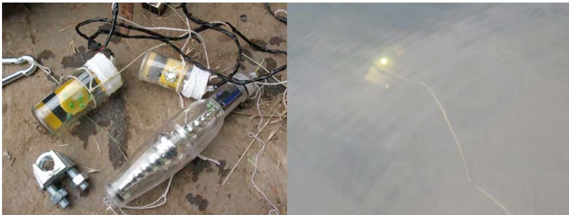
Left: Two Flishlight prototypes, above. Right: WLED Flishlight in underwater test.
