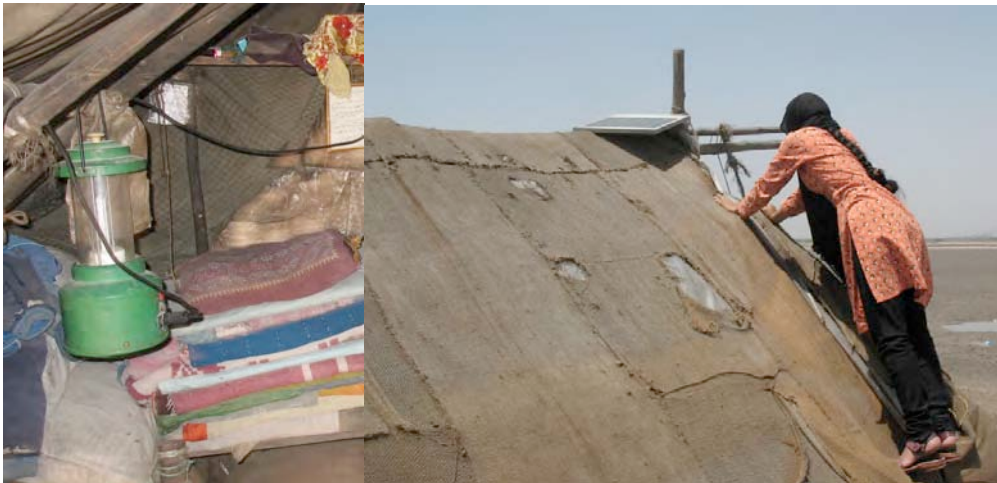
(Left) Local CFL Lantern found in fishing settlement, (Right), Adjusting solar panel for improved power supply and thus light output from CFL.
