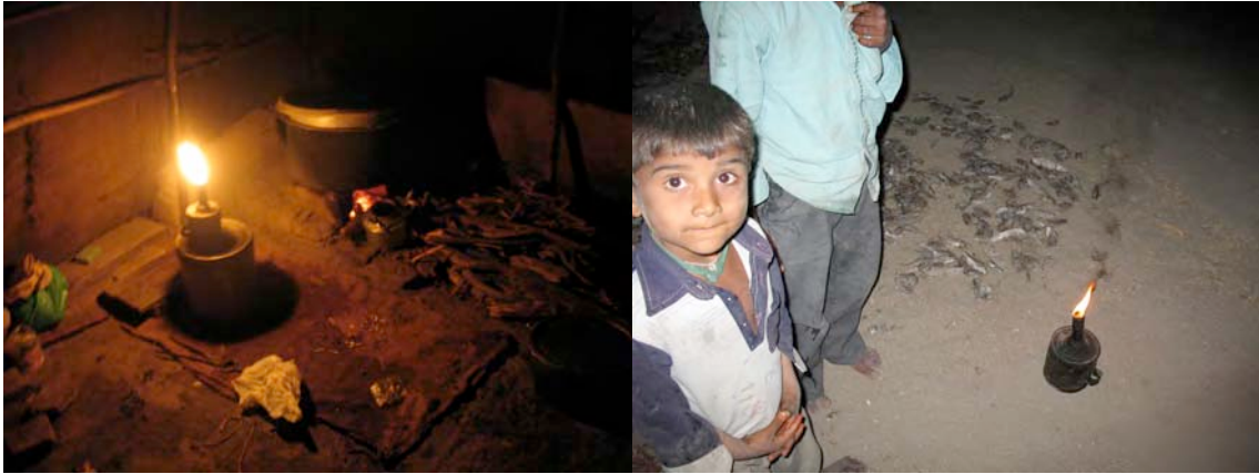
(Left) A “Chimney” seen indoors. 10-12 Lux were found on the brightest spot on the wall, lux levels of 2-3 lux were found towards the right edge of the rug in the center of the picture. Note that the lamp is elevated on a storage tin. (Right) Note the copious smoke produced by the Chimney.
