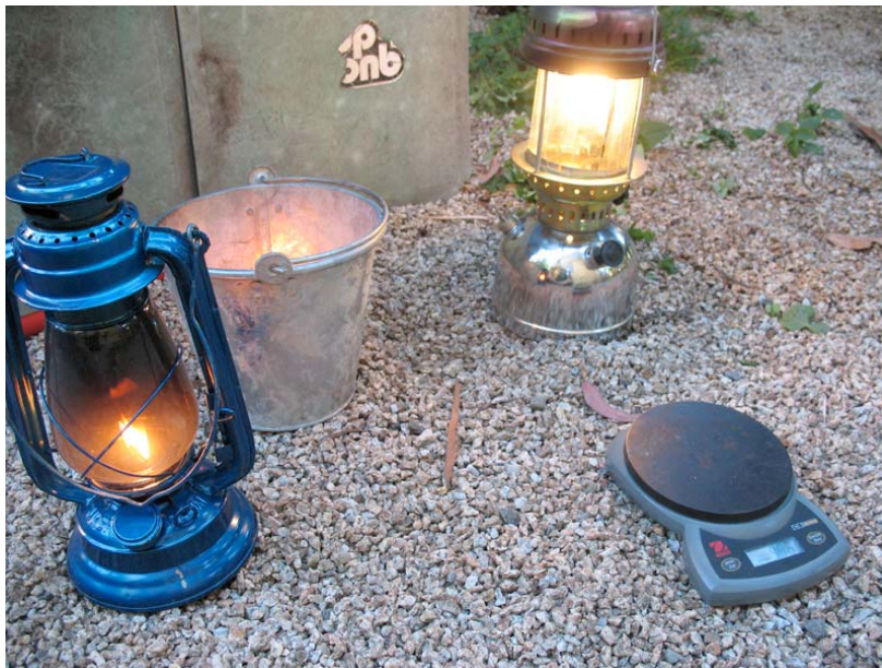
Fuel consumption testing of Kerosene lanterns in Berkeley, May 2007.
