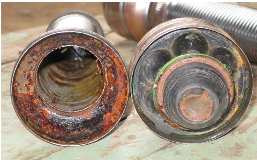
Photo 4. Corrosion from water and battery leakage.
