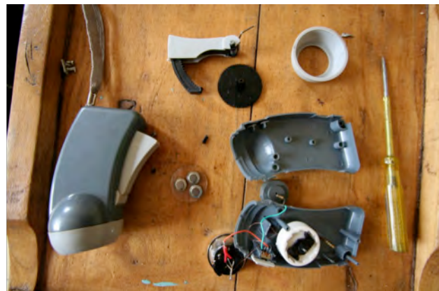
Figure 14. Counterfeit “crank-up” light using non-rechargeable coin batteries.
