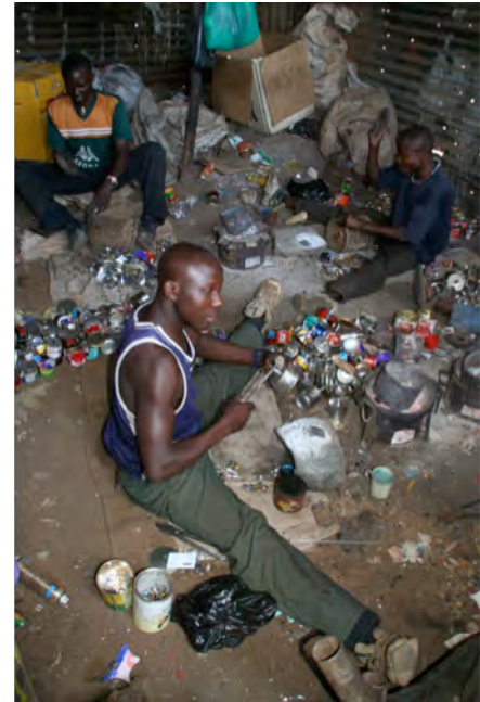
Figure 20. Cottage industry manufacture of “tin” lamps from discarded food cans in Kibera, Kenya. These products sell for $0.10 to $0.25 and can consume $50/year of kerosene, emitting 100 kg of CO 2 .
