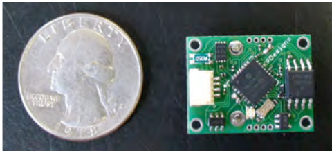
Figure 22. Micro-logger for monitoring on-time for off-grid LED lighting products. It includes the original "beta" version (above) and the current version of the microDL. Chart shows excerpt of data collected for one user in Kenya. For this particular trial, over 32 days of data collection the average LED lamp utilization (blue curve) was 2.6 hours per day. As battery loses charge in third night, light output can be seen to decrease. Logger designed by Kyle Palmer and others at Humboldt State University (HSU); photo/data gathered by Peter Johnstone at HSU.
