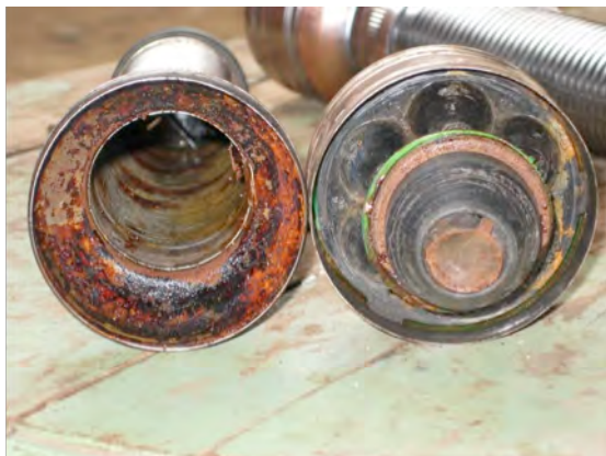
Figure 13. Example of LED lighting product made out of material that rusts (Photo: Jennifer Tracy)
