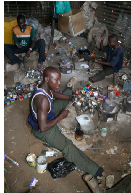
Figure 20. Cottage industry manufacture of “tin” lamps from discarded food cans in Kibera, Kenya. These products sell for $0.10 to $0.25 and can consumer $50/year of kerosene, emitting 100 kg of CO 2 .
