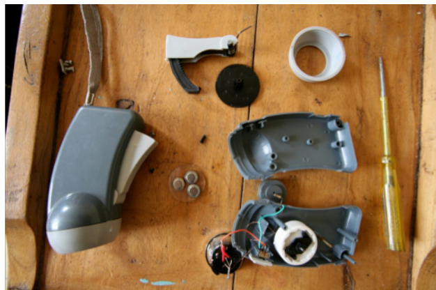
Figure 14. Counterfeit “crank-up” light using non-rechargeable coin batteries.
